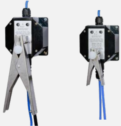
The Earth-Rite MULTIPOINT II's energy efficient remote indicator stations provide ground status indication for each individual channel. The attention grabbing high intensity GREEN LED pulses continuously when a positive ground connection is made.
