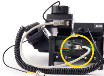
4. Connect the D-sub connector and the antenna cable.
