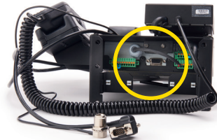
2. Undo antenna cable and D-sub connector.
