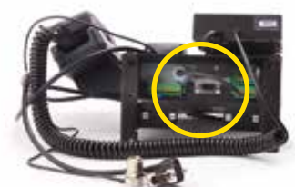
2. Undo antenna cable and D-sub connector.
