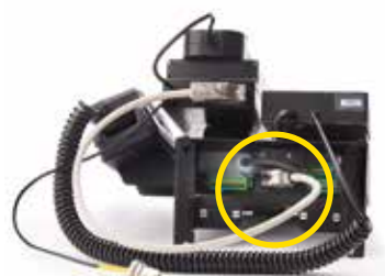
4. Connect the D-sub connector and the antenna cable.
