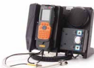
3. Mount the bayonet bracket for the Cradle kit SED.
