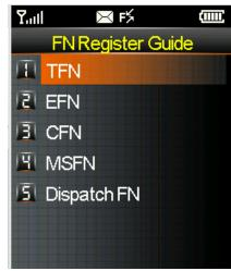
Choose **TFN** to display the function number registration page. After you enter relevant information, press the **OK** key. In the case of the train shunting mode, enter five-digit train number (pad zeros if the train number has less than five digits).
