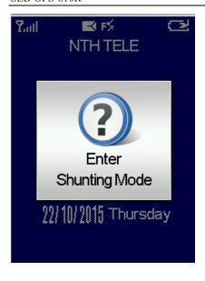
In the standby state, press . The UI asking whether to enter the shunting mode is displayed.
