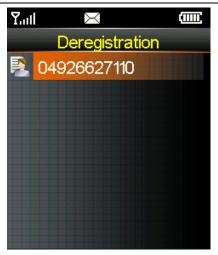
Press the **OK** key to display the main menu, choose **Identity>Deregistration** to display the deregister the function number UI, and press the **OK** key.
