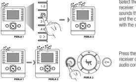
Select the desired indoor receiver. The calling receiver sounds the line-free tone and the called receiver rings with the chosen ringtone.
