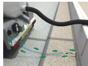
Continuous Ground Loop Monitoring check
