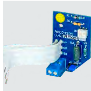
I.S Switching PCB Product Code: ER2/IS/KIT
