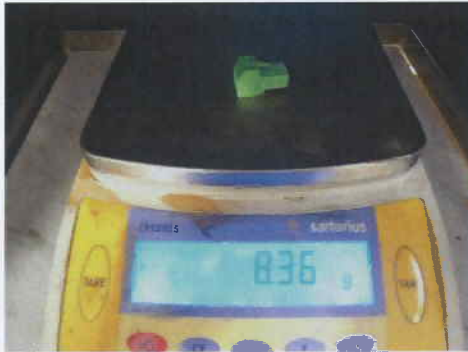
Photo 7: Phoenix Contact PC4/2-ST-7, 8.4 g.
