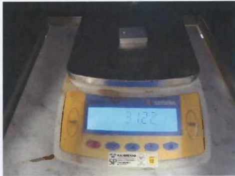
Photo 13: Transformer heat sink, 31.2 g.
