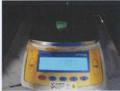
Photo 8: Phoenix Contact PC4/2-ST-7 3.0 g.
