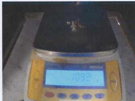
Photo 6: Metal parts from Phoenix Contact PC4/4-ST, 10.9 g.
