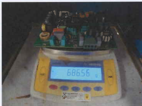
Photo 15: PCB with electronic device, 686.6 g.
